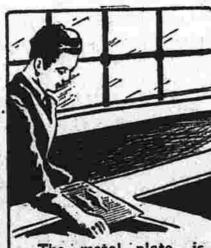
The metal plate is placed in an acid bath which eats away the metal around the dots. The dots have been made impervious to the acid by the resist.
